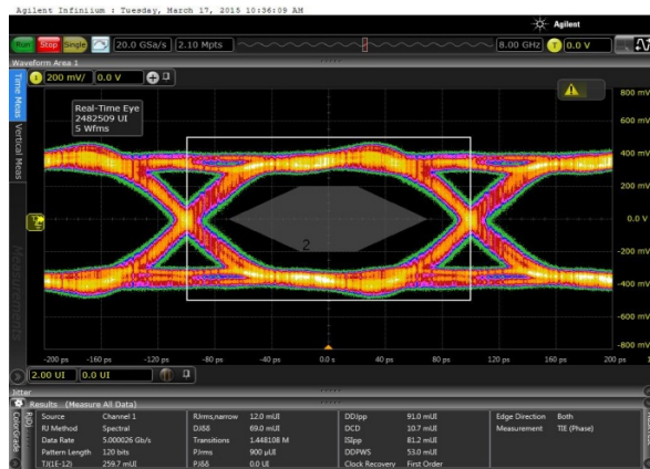
Figure 86. Eye at 5-Gbps Bit Rate with Default Output Swing
