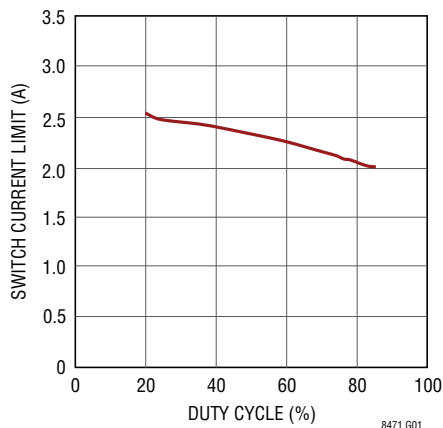
Primary Switch Current Limit at 500kHz
