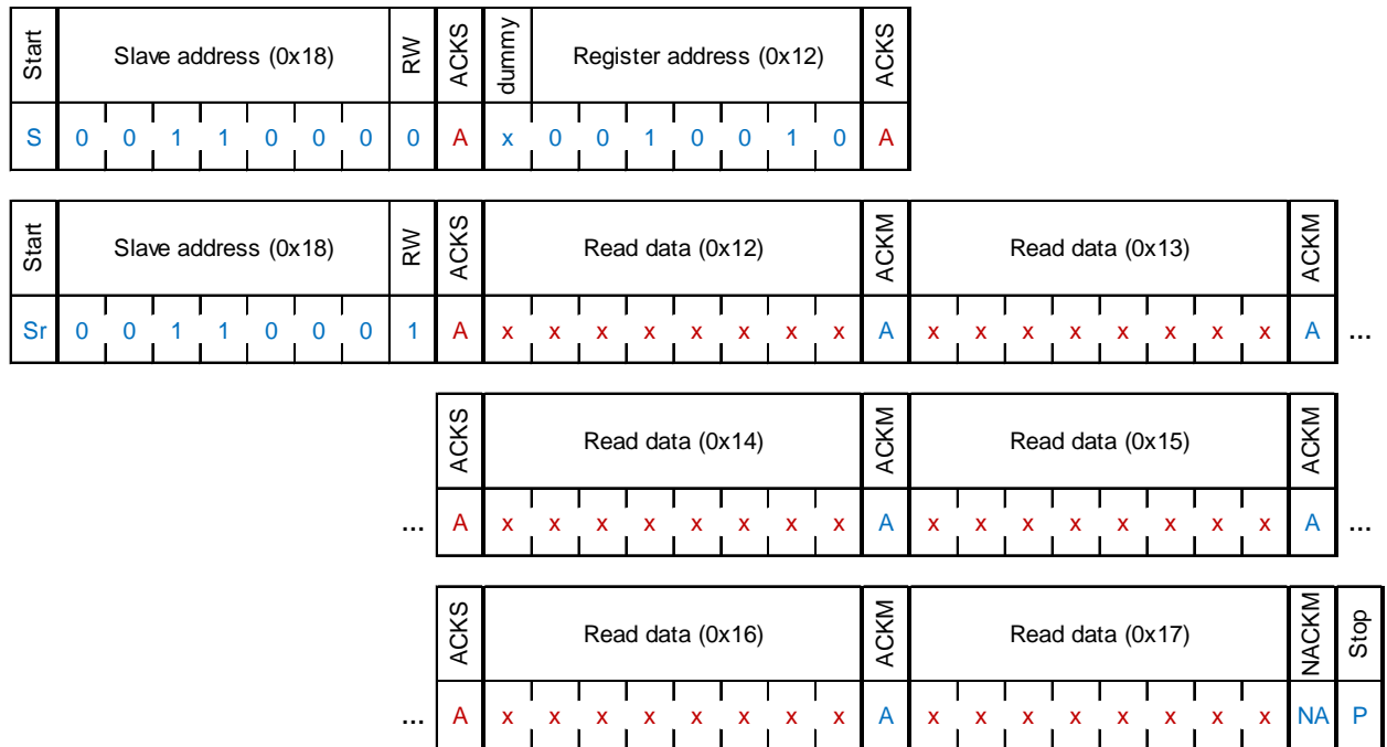
Figure 5: I 2 C multiple read
