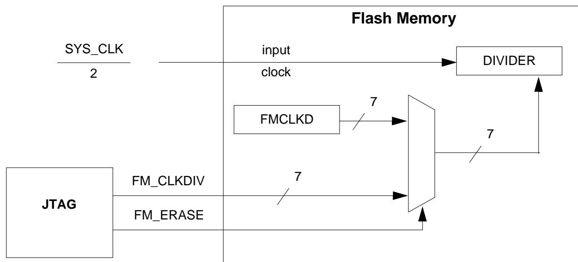
**Figure 7-1 JTAG to FM Connection for Lockout Recovery**
