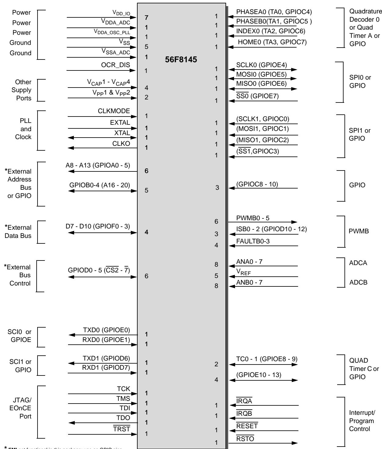
**Figure 2-2 56F8145 Signals Identified by Functional Group<sup>1</sup> (128-Pin LQFP)**
