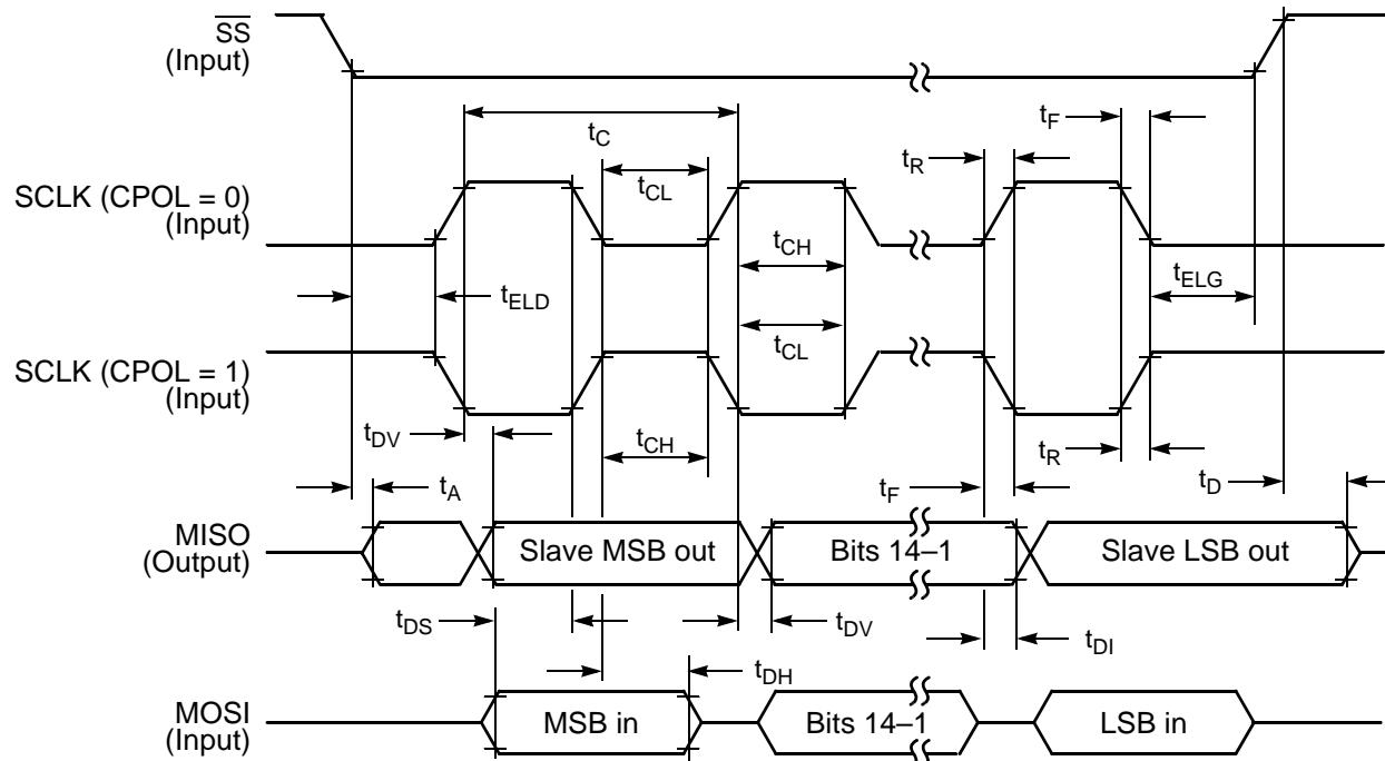
Figure 10-12 SPI Slave Timing (CPHA = 1)
