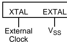
Note: When using an external clocking source with this configuration, the input "CLKMODE" should be high and COHL bit in the OSCTL register should be set to 1.
