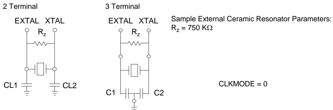
Figure 3-3 Connecting a Ceramic Resonator
