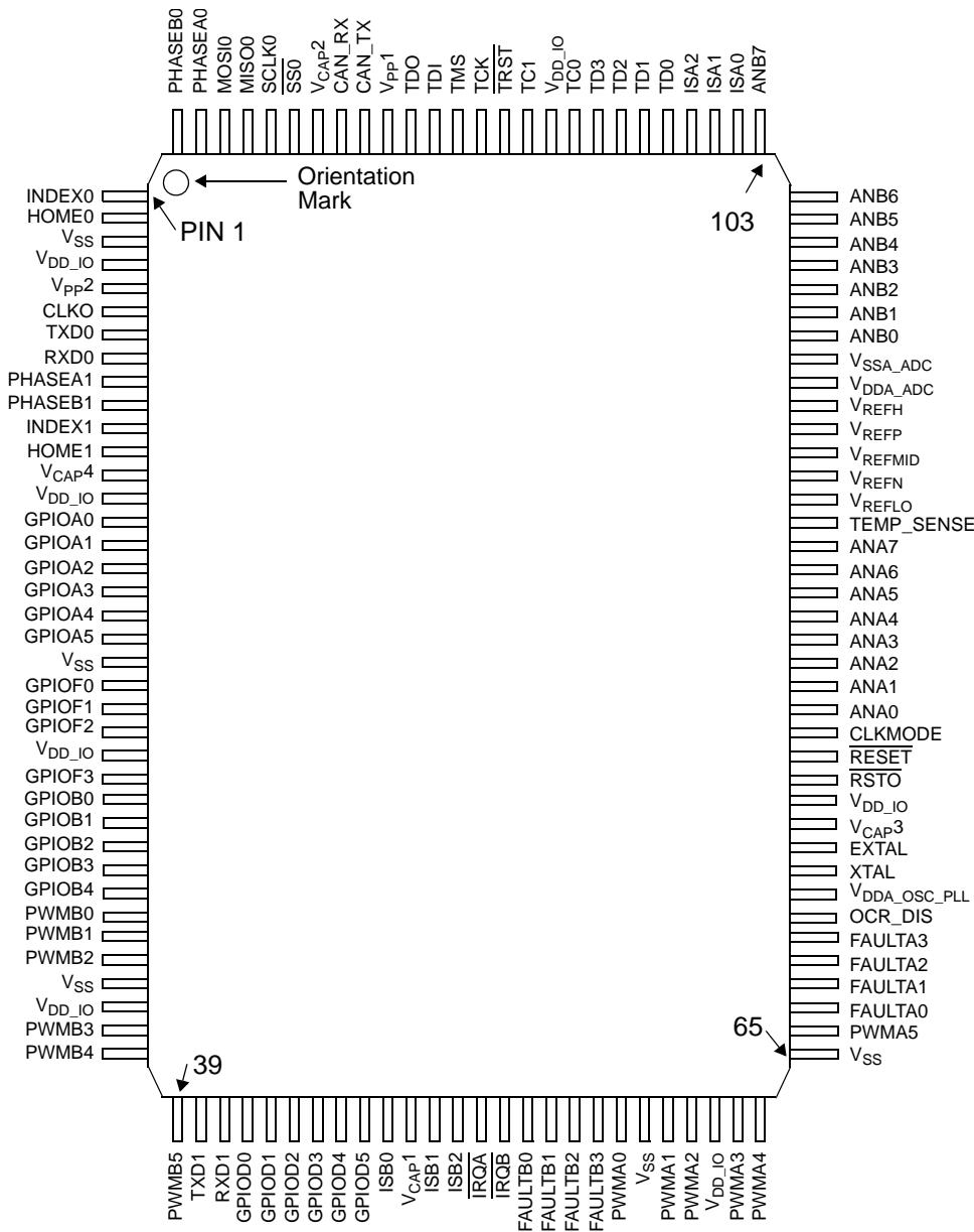
**Figure 11-1 Top View, 56F8345 128-pin LQFP Package**
