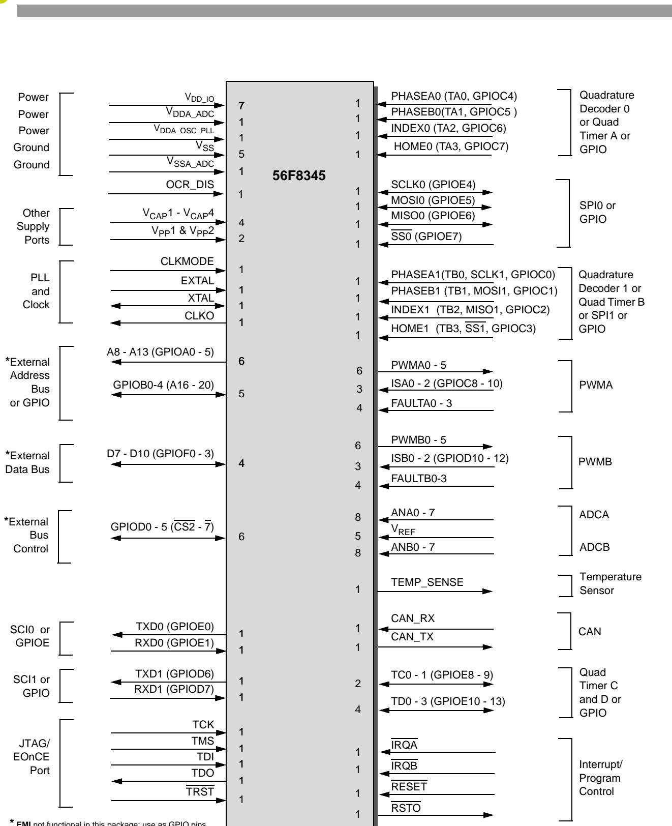
**Figure 2-1 56F8345 Signals Identified by Functional Group<sup>1</sup> (128-Pin LQFP)**
