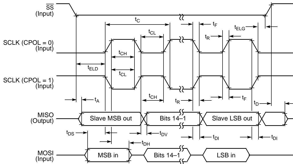
Figure 10-11 SPI Slave Timing (CPHA = 0)
