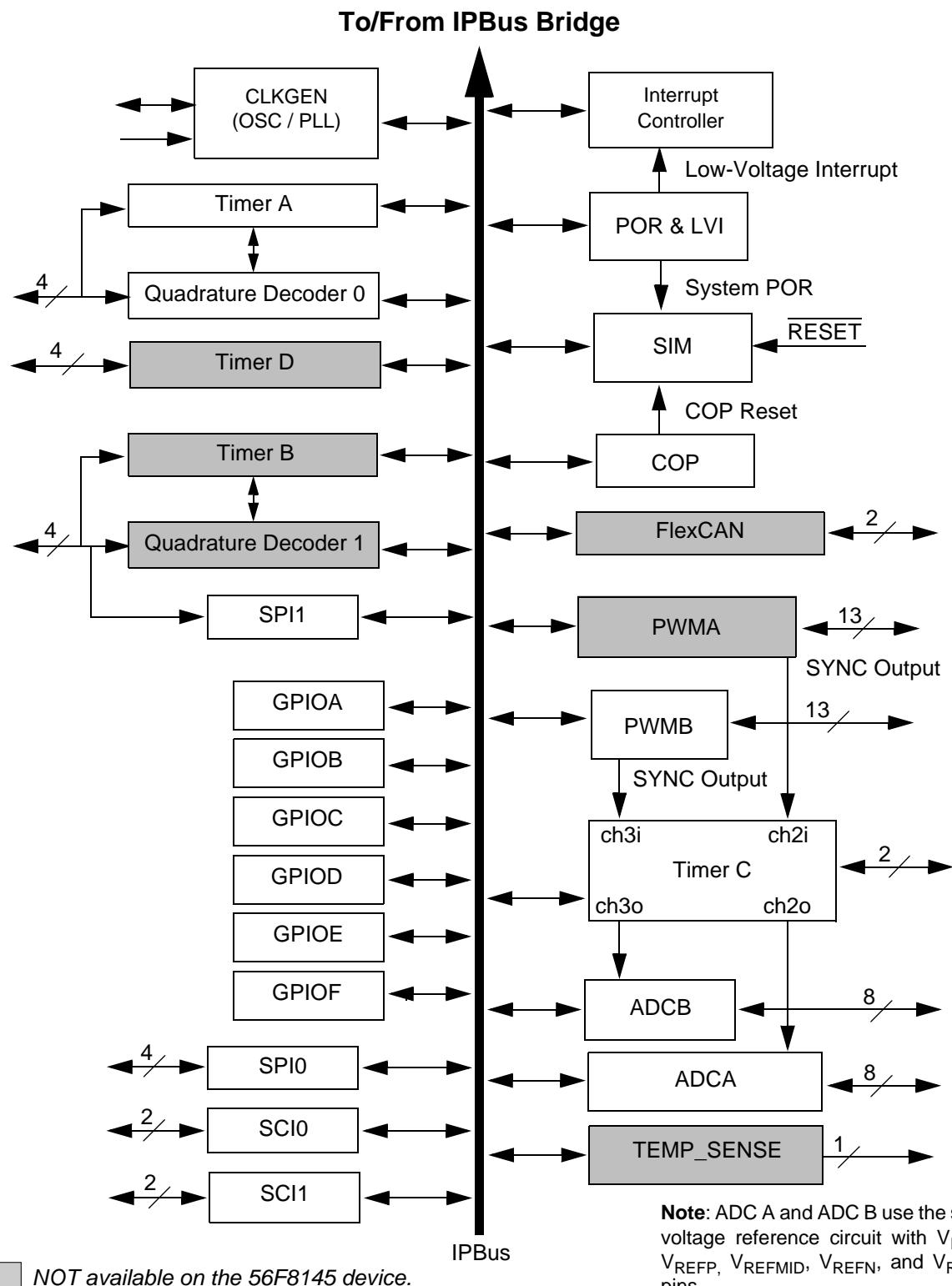
**Note:** ADC A and ADC B use the same voltage reference circuit with  $V_{REFH}$ ,  $V_{REFP}$ ,  $V_{REFMID}$ ,  $V_{REFN}$ , and  $V_{REFLO}$  pins.
