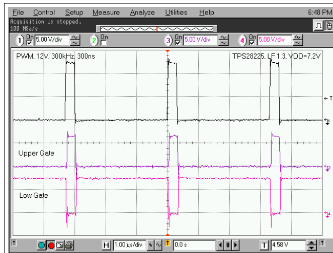
Figure 23. 12-V PWM Pulse at V_{DD} = 7.2 V
