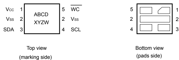
Figure 3. UFDFPN5 (DFN5) package connections
