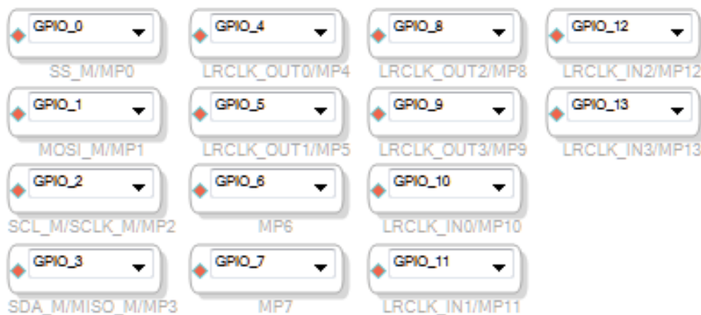
Figure 76. Complete Set of General-Purpose Outputs in SigmaStudio
