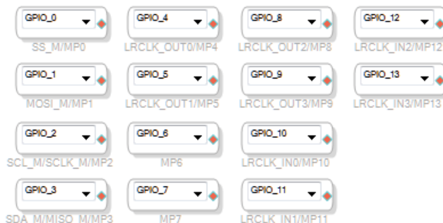
Figure 75. Complete Set of General-Purpose Inputs in SigmaStudio
