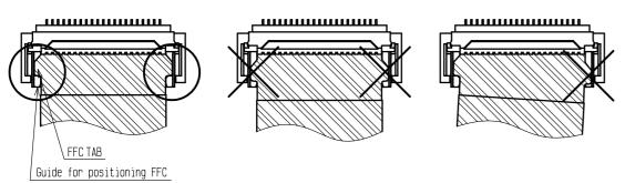
♦ Checking the Locking Condition
