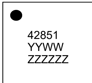
Figure 26. Top Marking Specification
