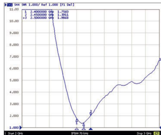
Antenna VSWR on Test Board
