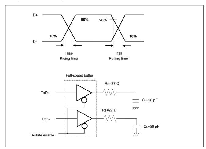
6. USB Full-speed connection is performed via twist pair cable shield with 90  $\Omega$  ± 15% characteristic impedance (Differential Mode).
