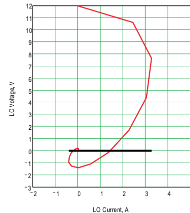
Figure 25. Turnoff Voltage and Current Switching Diagram
