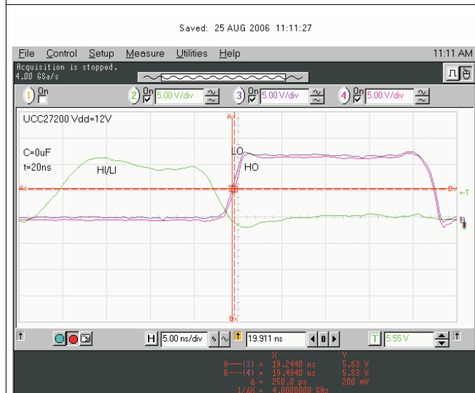
Figure 32. 20-ns Input Pulse Delay Matching
