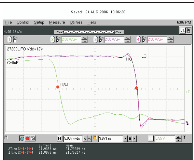
Figure 31. V LO and V HO Falling Edge Delay Matching
