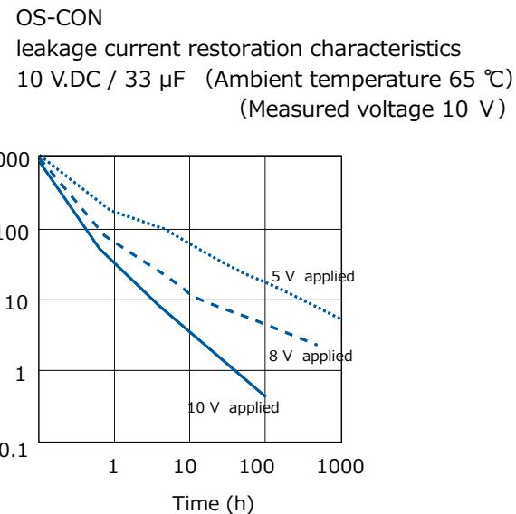
※ To make the recovery of LC values easy to show, samples that LC values have been increased on purpose are used in the test.
