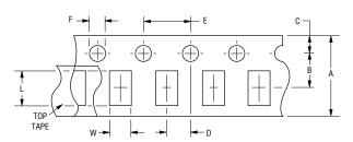
NOTES: TAPE MATERIAL IS PAPER. TAPE THICKNESS IS:  $\frac{0.6\pm0.03}{(0.024\pm0.0012)}$  COVER TAPE ADHESION IS 35  $\pm25$  GRAMS.
